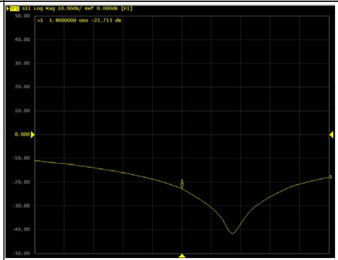
Return Loss Test- Body
