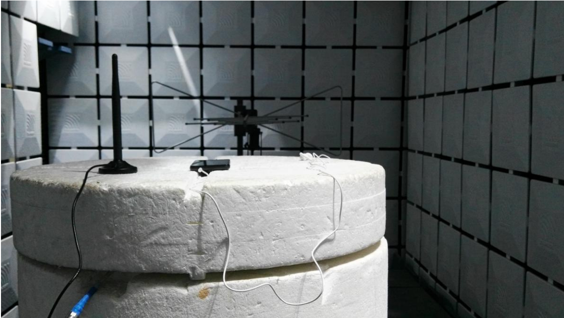
Radiated Spurious Emission (below 1GHz)
