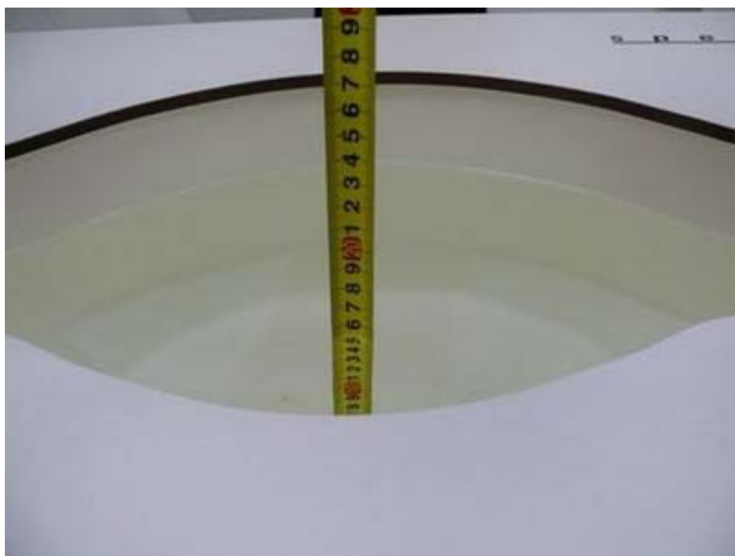
Picture 8: Liquid depth in the flat Phantom (2450 MHz, 15.3cm depth)
