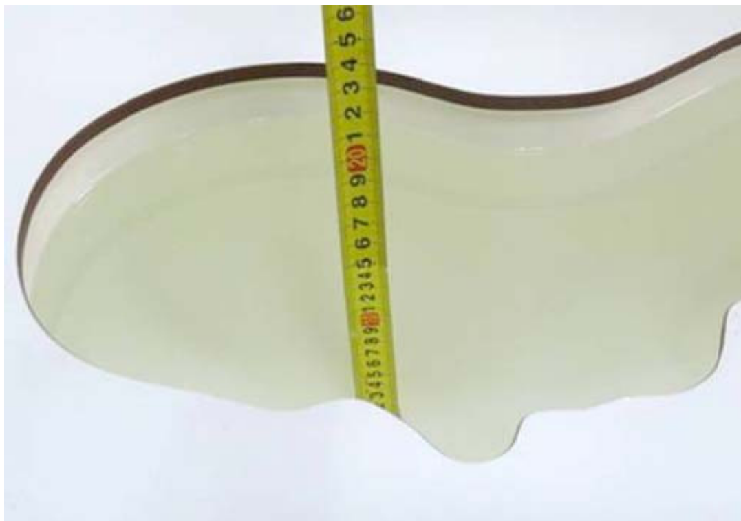
Picture 7: Liquid depth in the head Phantom (2450 MHz, 15.4cm depth)
