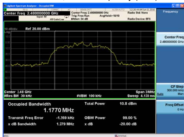
BT 2DH5 CH78, Carrier frequency (MHz): 2480
