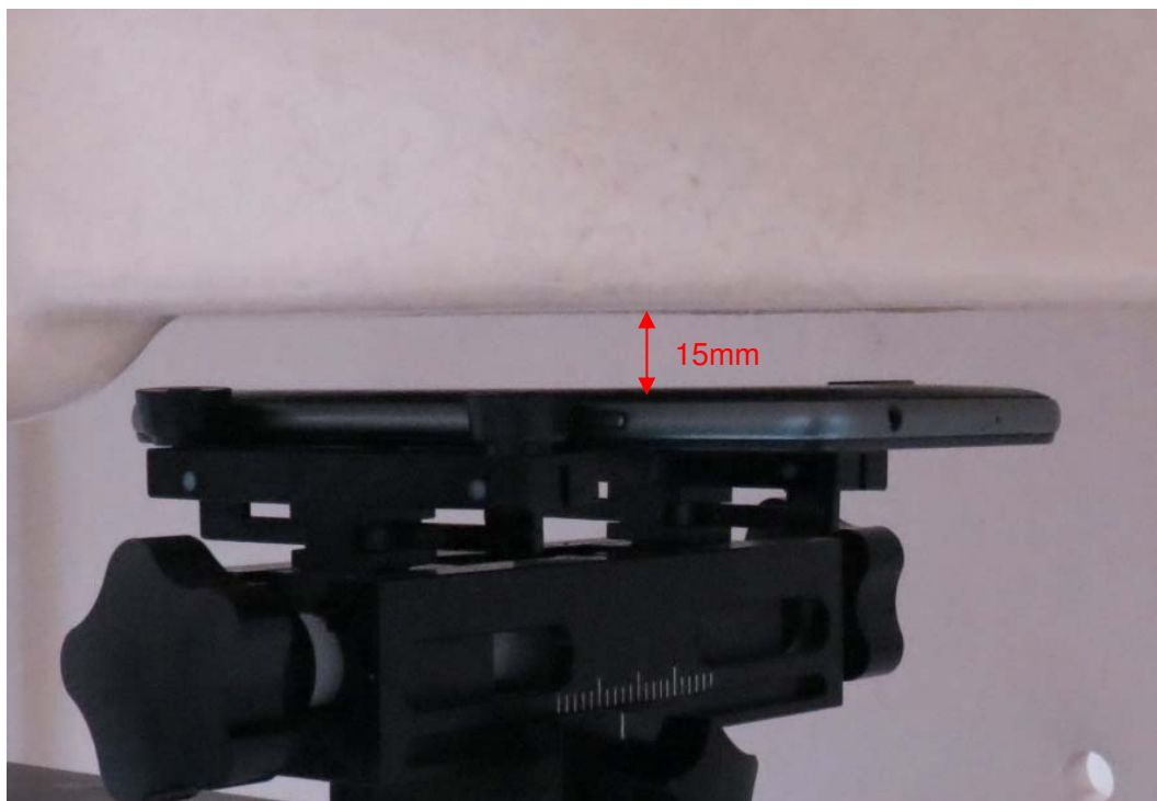
Picture 6: Back Side, the distance from handset to the bottom of the Phantom is 15mm
