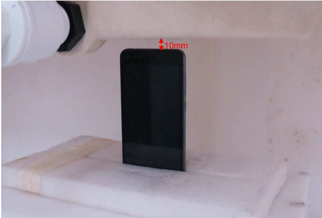
Picture 12: Top Side, the distance from handset to the bottom of the Phantom is 10mm
