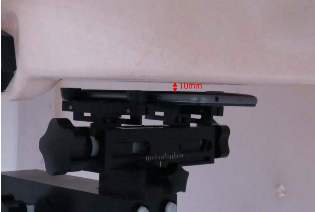
Picture 8: Back Side, the distance from handset to the bottom of the Phantom is 10mm
