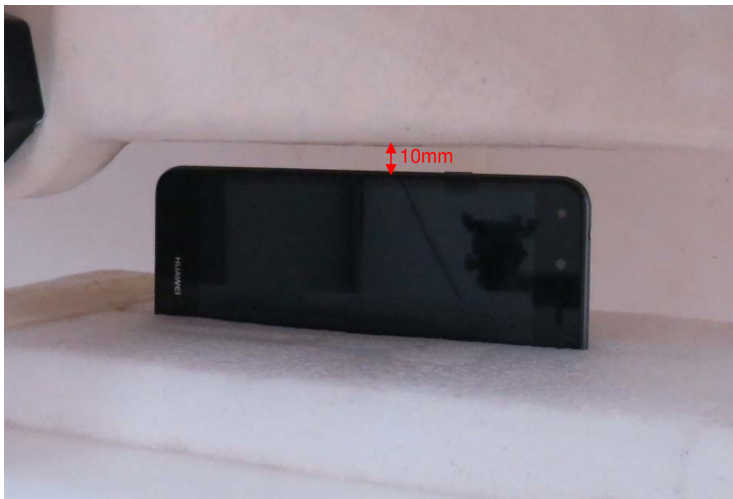
Picture 10: Left Side, the distance from handset to the bottom of the Phantom is 10mm
