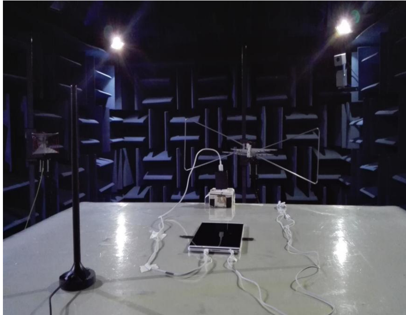
Radiated Spurious Emission (1GHz to18GHz)
