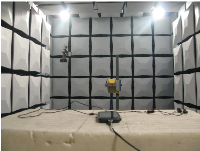
Radiated Spurious Emission (3GHz to18GHz)
