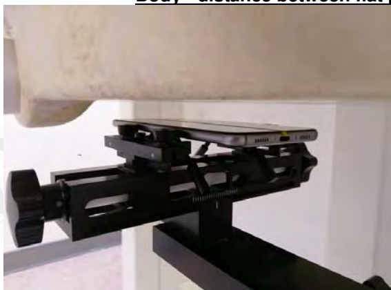
Fig.7 EUT Front side to flat phantom
