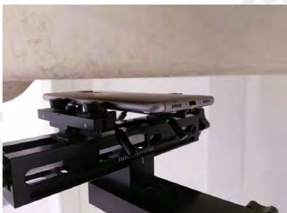
Fig.8 EUT Back side to flat phantom
