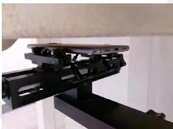
Fig.11 EUT Back side to flat phantom
