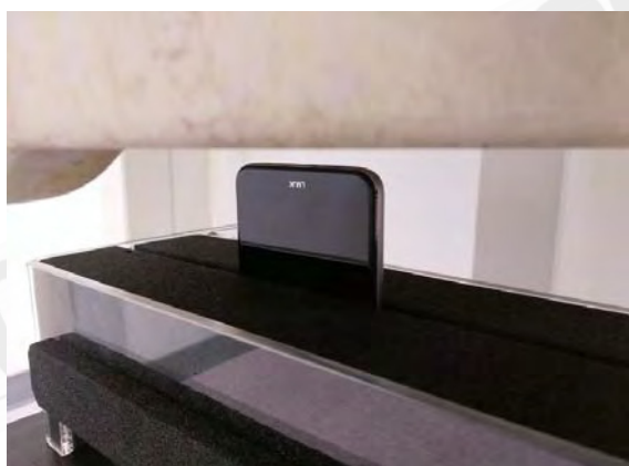
Fig.10 EUT Bottom side to flat phantom
