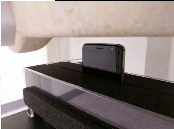
Fig.12 EUT Top side to flat phantom
