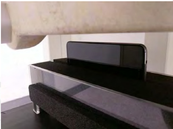
Fig.13 EUT Left side to flat phantom
