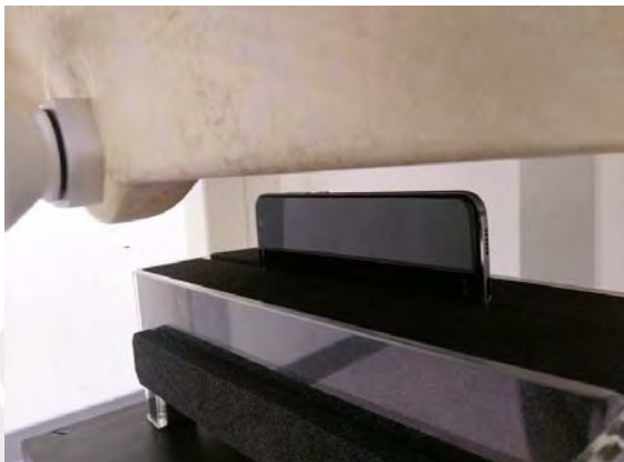
Fig.14 EUT Right side to flat phantom
