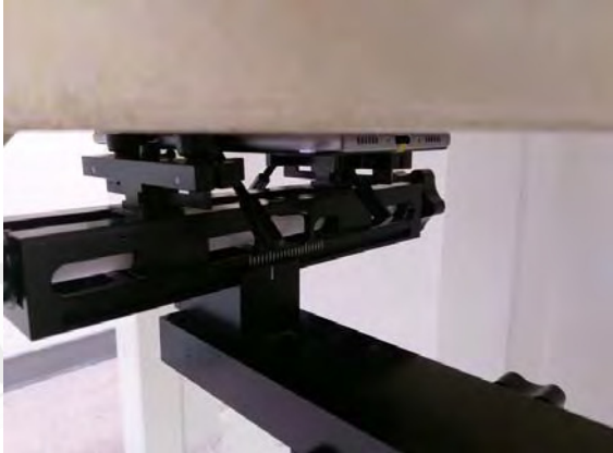
Fig.15 EUT Back side to flat phantom
