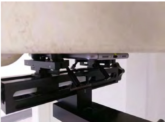
Fig.17 EUT Front side to flat phantom
