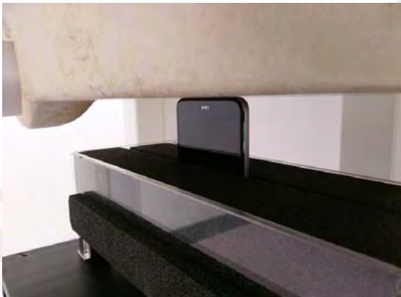
Fig.16 EUT Bottom side to flat phantom
