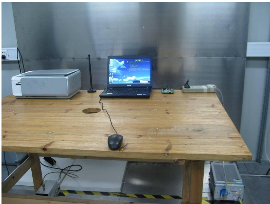
Conducted Emissions for AC Power
