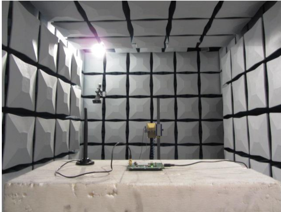
Radiated Spurious Emission (3GHz to18GHz)
