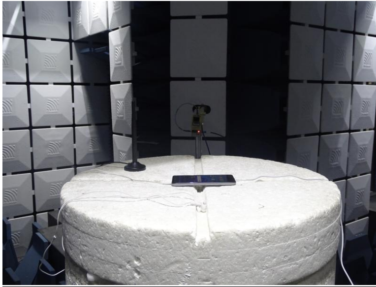
Radiated Spurious Emission (18GHz to26.5GHz))
