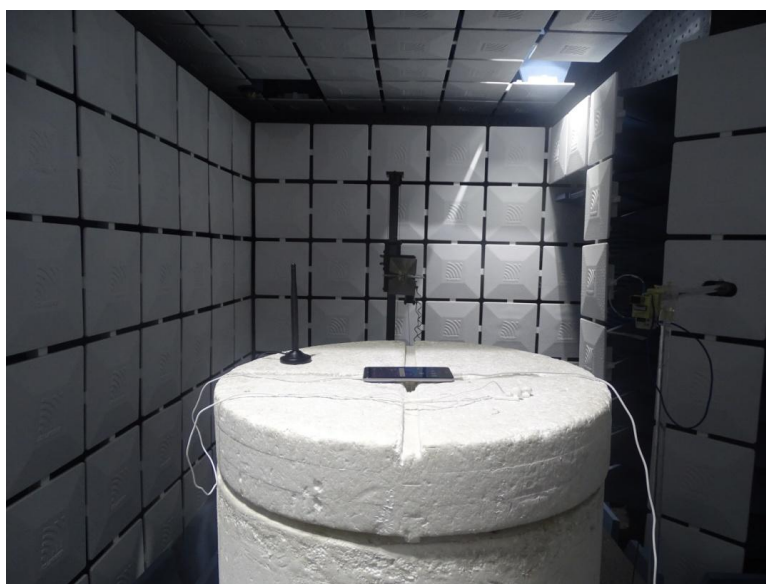
Radiated Spurious Emission (3GHz to18GHz)
