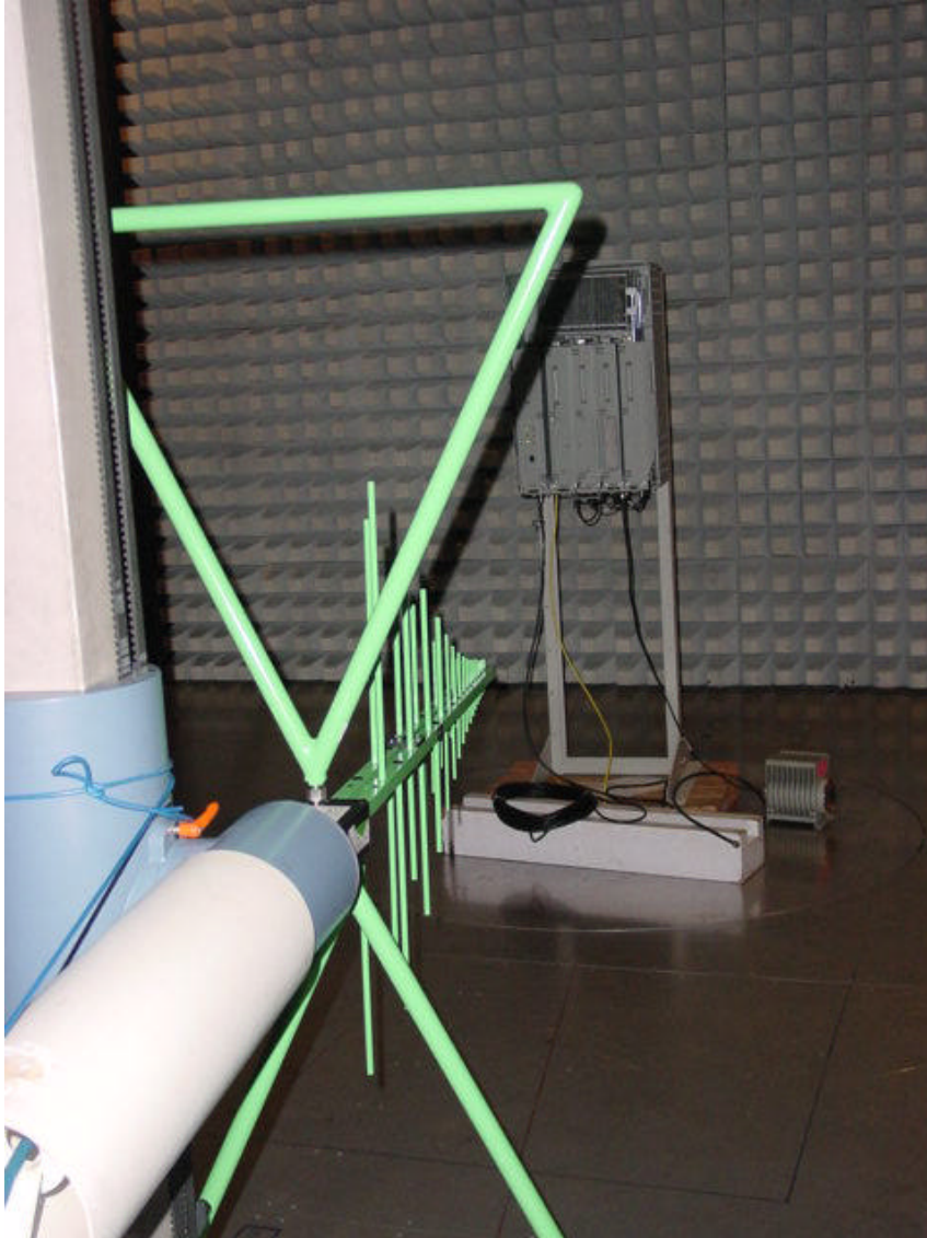
Photo ERP Measurement 30 MHz – 1 GHz
