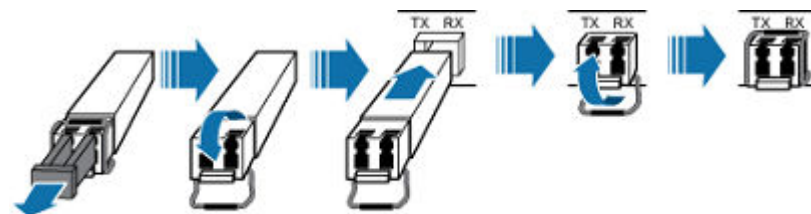
Figure 5-5 Installing the new optical module
