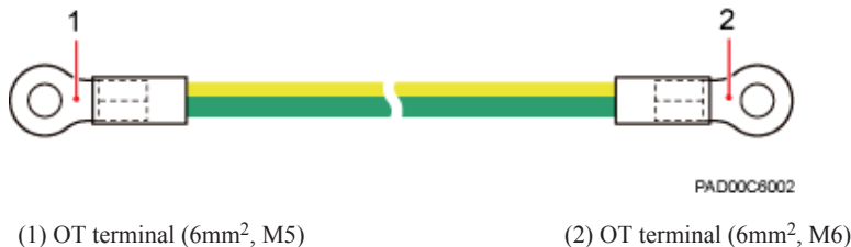
Figure 14-39 Exterior of a PGND cable
