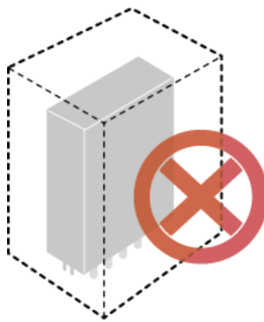
Figure 9-1 Inappropriately installed pRRU
