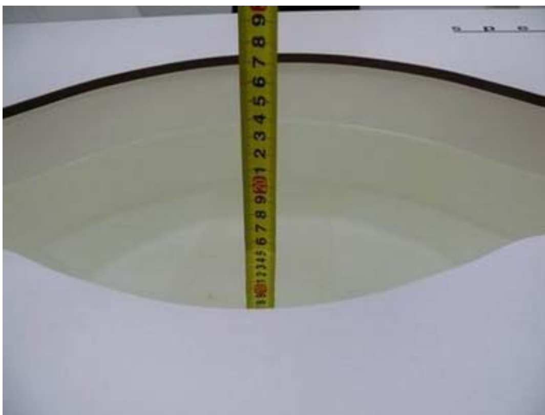
Picture 4: Liquid depth in the flat Phantom (1900 MHz, 15.2cm depth)
