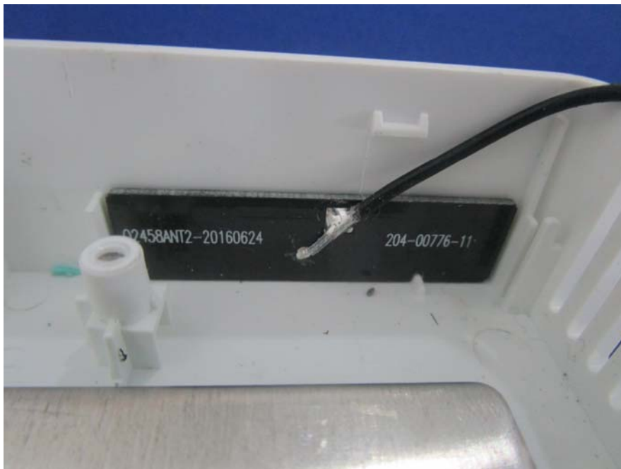
EUT – Wifi Antenna View
