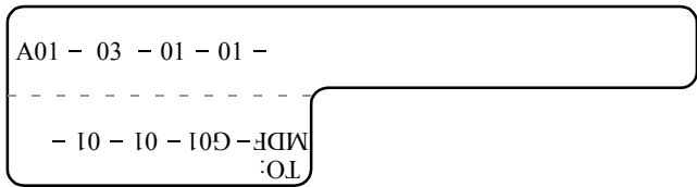
Figure 5-92 Sample label on a user cable
