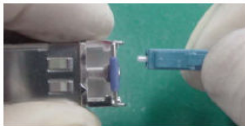
Figure 5-98 Using fibers to protect an optical module
