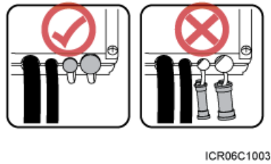
Figure 8-21 Correct placement of waterproof blocks
