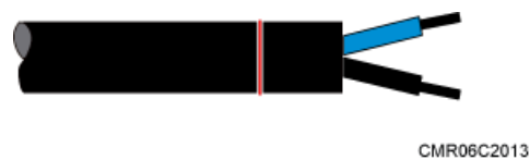
Figure 11-4 Stripping the sheath off each core wire
