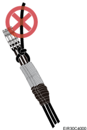
Figure 6-6 Incorrect binding method
