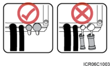
Figure 8-21 Correct placement of waterproof blocks
