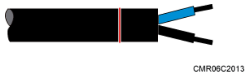
Figure 11-4 Stripping the sheath off each core wire
