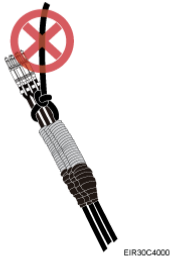
Figure 6-6 Incorrect binding method
