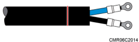
Figure 11-5 Adding OT terminals
