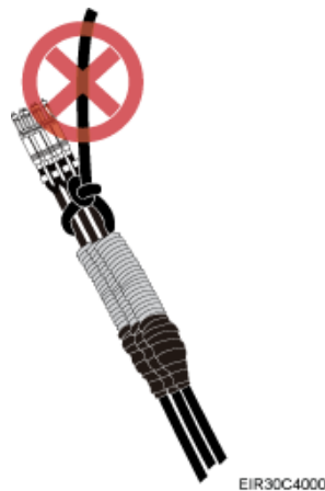
Figure 7-8 Incorrect binding method
