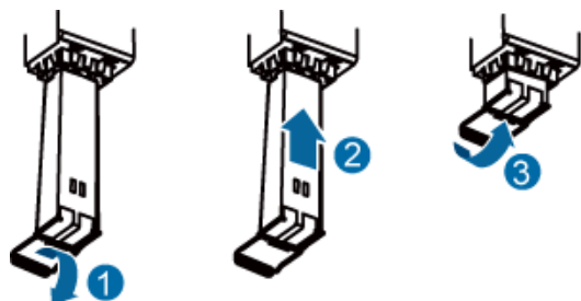
Figure 9-26 Installing an optical module
