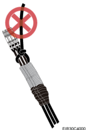
Figure 7-8 Incorrect binding method
