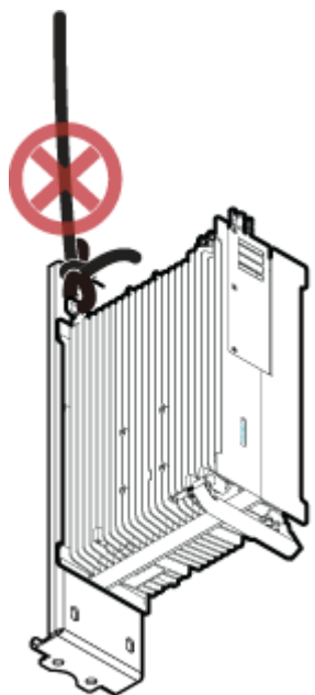
Figure 6-12 Incorrect binding method (2)
