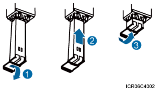
Figure 7-23 Installing an optical module
