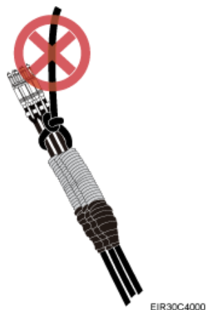
Figure 6-8 Incorrect binding method
