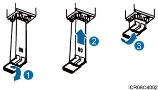
Figure 7-25 Installing an optical module
