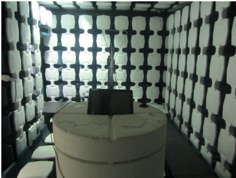
Radiated Spurious Emission (below 3GHz)
