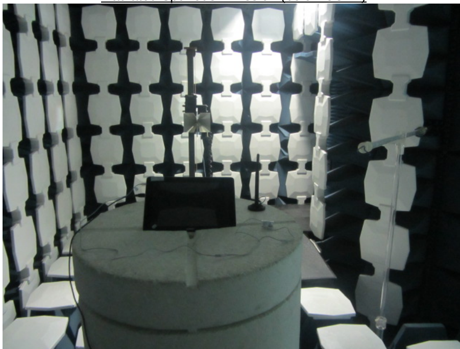
Radiated Spurious Emission (3GHz to18GHz)
