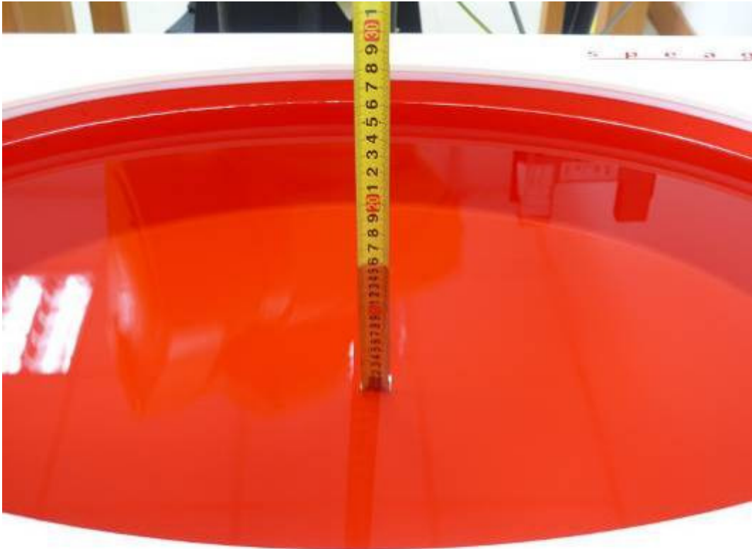
Picture 14: Liquid depth in the flat Phantom (5600 MHz, 15.3cm depth)
