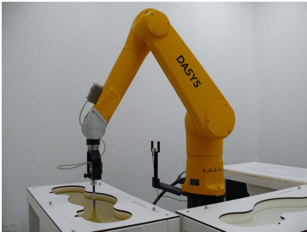
Picture 1: Specific Absorption Rate Test Layout
