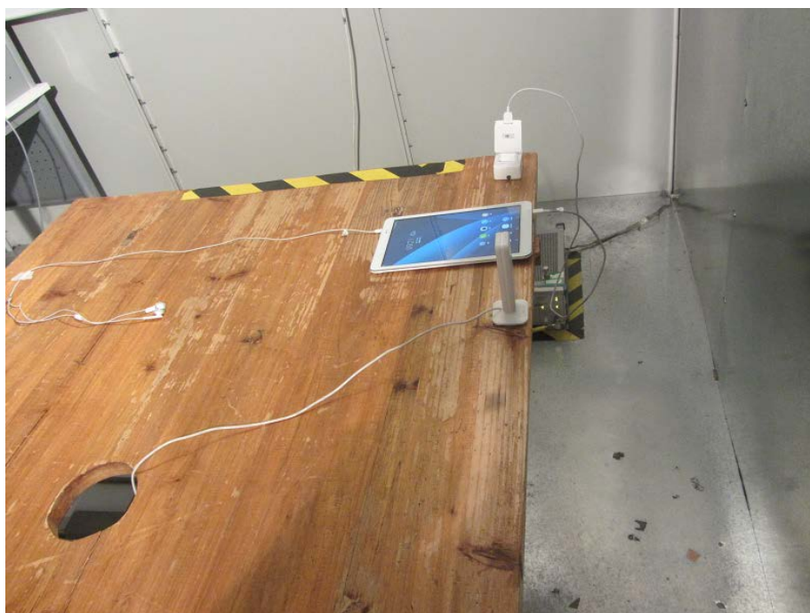
Conducted Emissions with AC Ports
