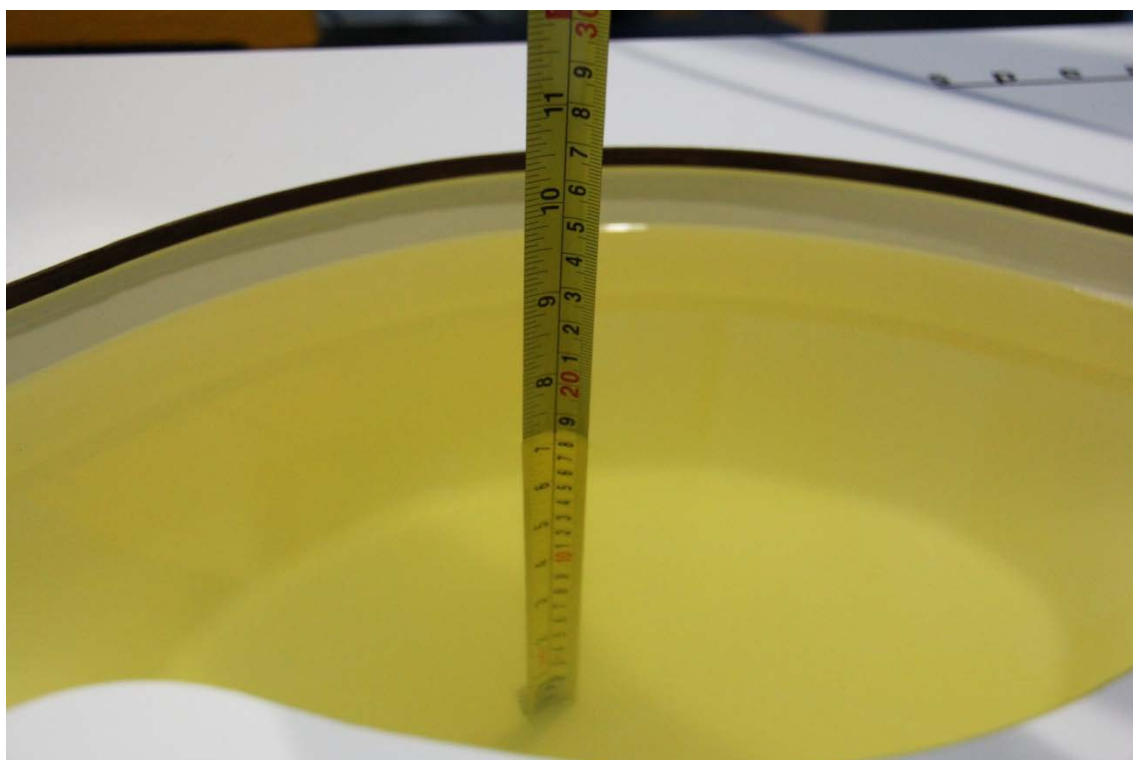
Picture 7-10 Liquid depth in the Flat Phantom (2450MHz)
