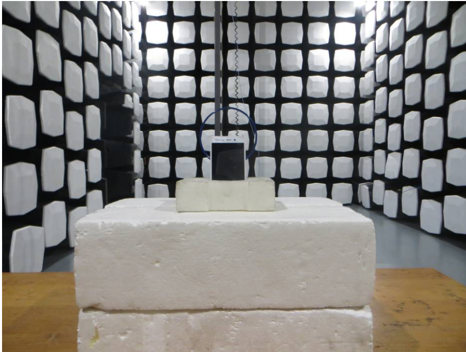
5. Radiated Emissions (Part 15C) (below 30MHz)
