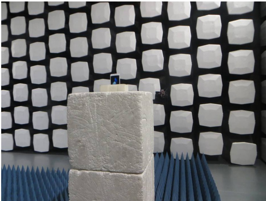
10. Radiated Emissions (Part 22/24) (Above 3GHz)
