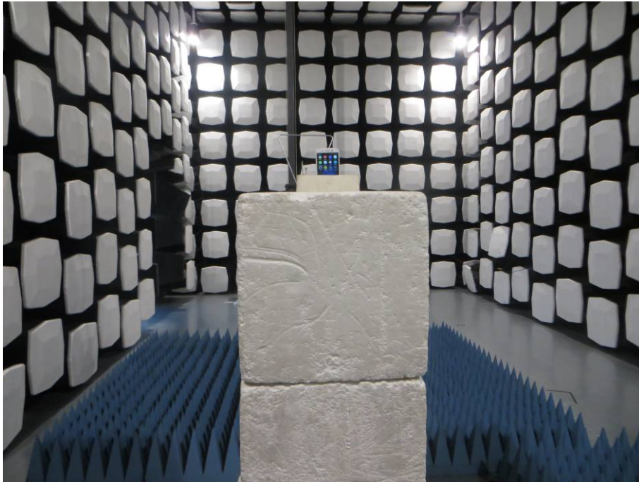
9. Radiated Emissions (Part 22/24) (below 3GHz)
