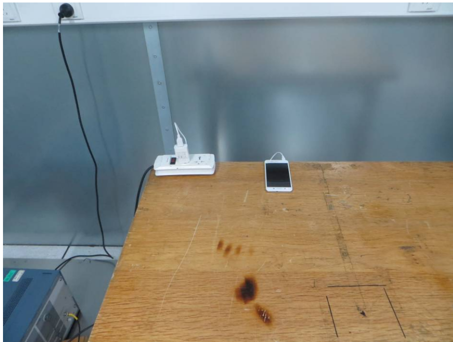
14. Conducted Emission (Part 15B Charging mode)
