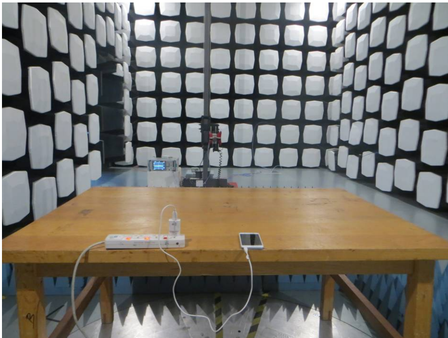
4. Radiated Emissions (Part 15B Charging mode) (Above 1GHz)
