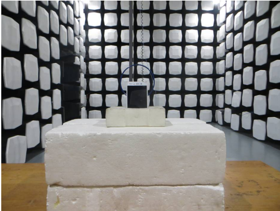
5. Radiated Emissions (Part 15C) (below 30MHz)
