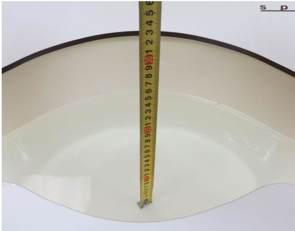
Picture 5: Liquid depth in the flat Phantom (5800 MHz, 10.3cm depth)
