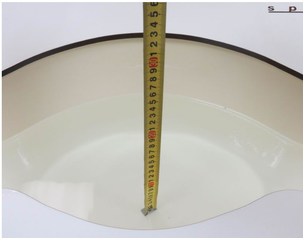
Picture 4: Liquid depth in the flat Phantom (5200 MHz, 10.3cm depth)
