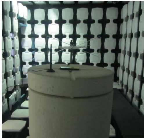
Radiated Spurious Emission (below 3GHz)
