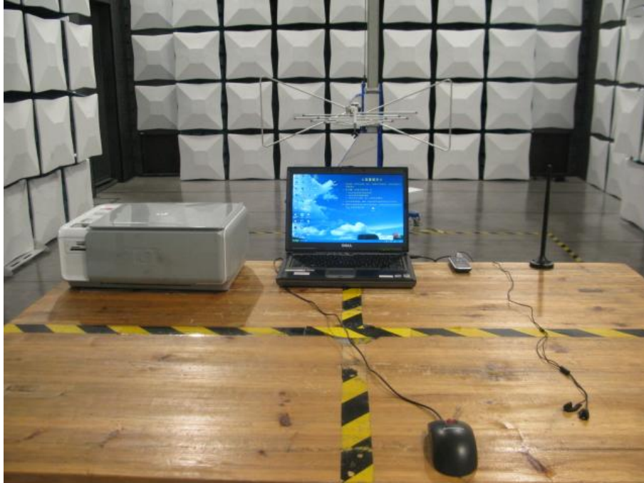
Radiated Spurious Emission (below 1GHz)
