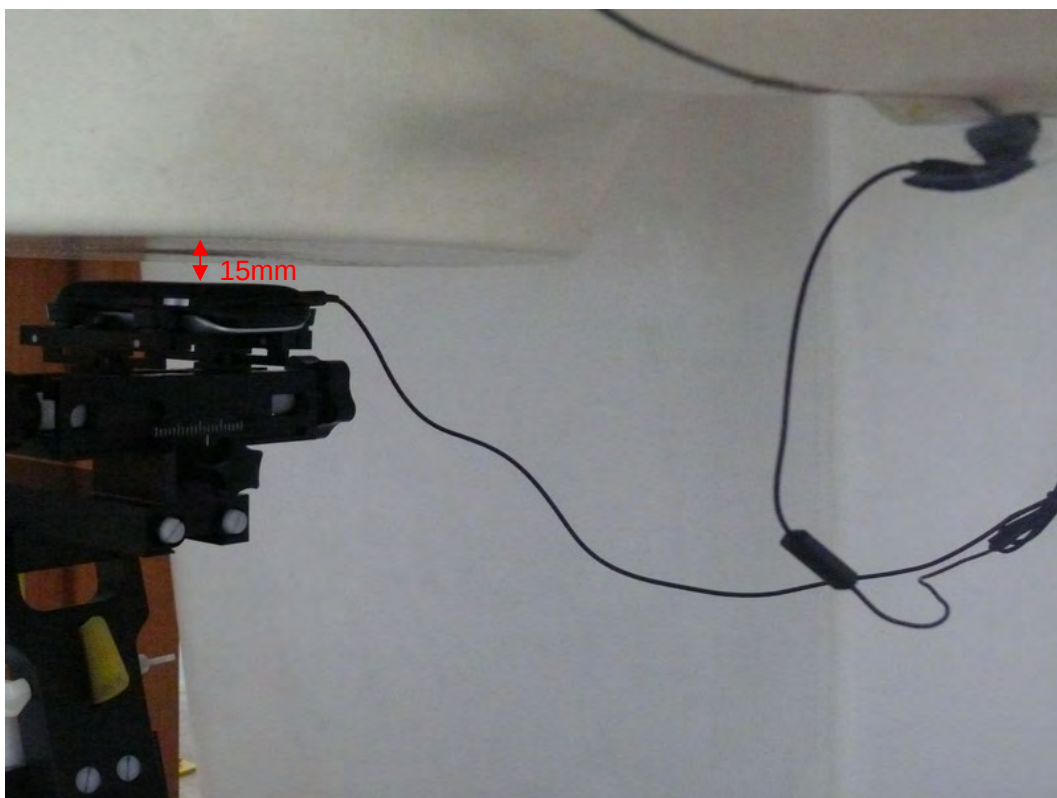
Picture 16: Body with earphone, The EUT display towards ground, the distance from handset to the bottom of the Phantom is 15mm (Cover Closed)
