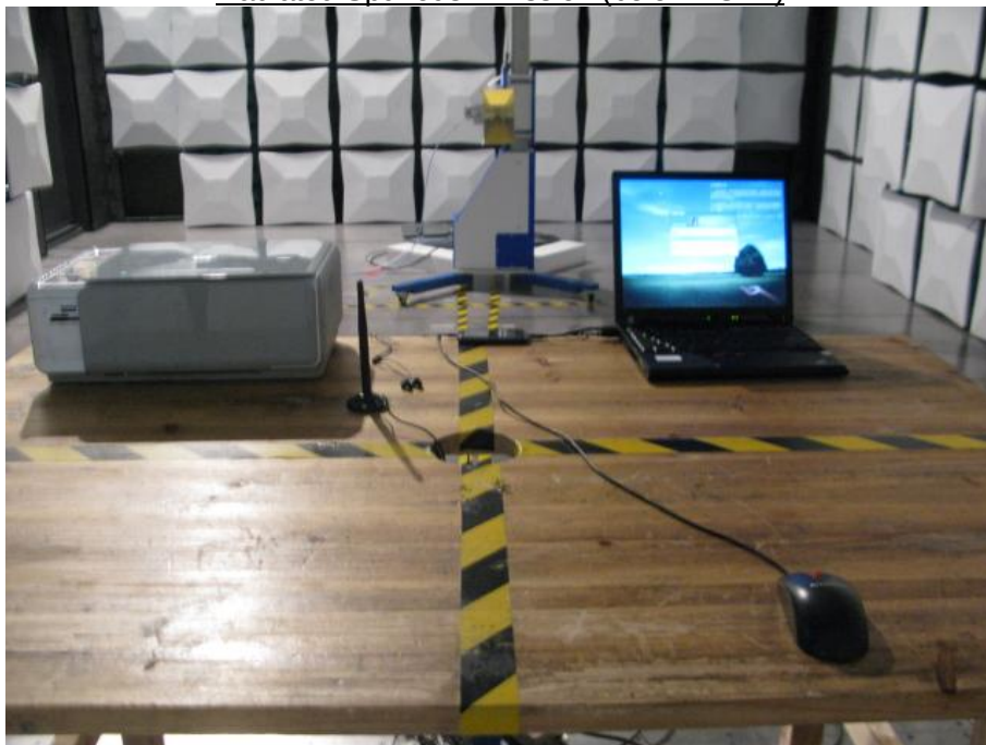
Radiated Spurious Emission (1GHz to 18GHz)
