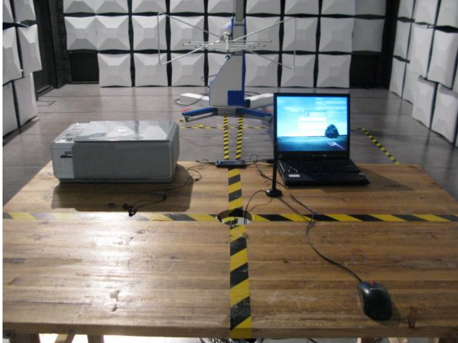
Radiated Spurious Emission (below 1GHz)
