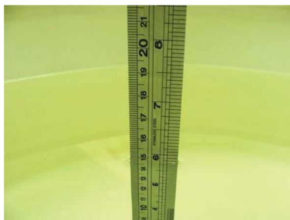
Fig 6.2 Photo of Liquid Height for Body SAR
