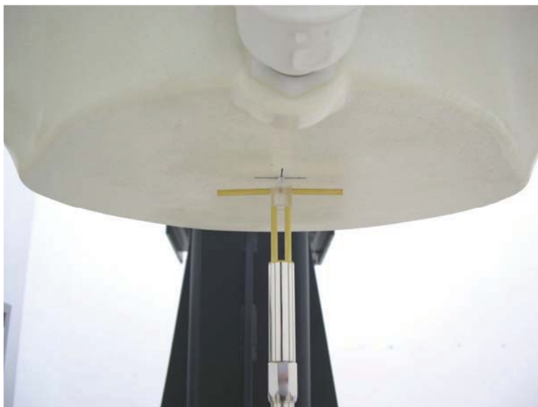
Fig 8.2 Photo of Dipole Setup
