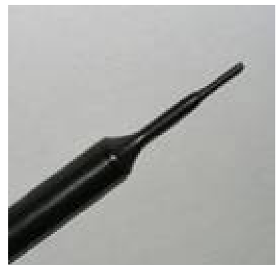
Figure 2. EX3DV4 E-field Probe
