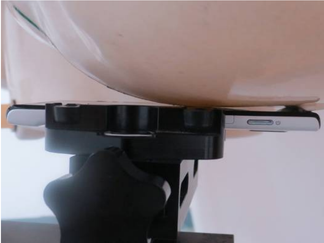
Picture 11: Left Hand Touch Cheek Position
