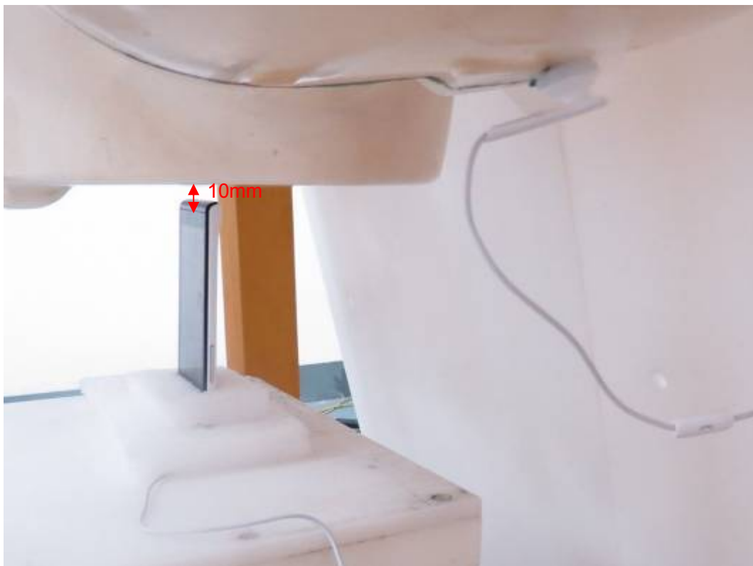
Picture 22: Bottom Edge with earphone, the distance from handset to the bottom of the Phantom is 10mm
