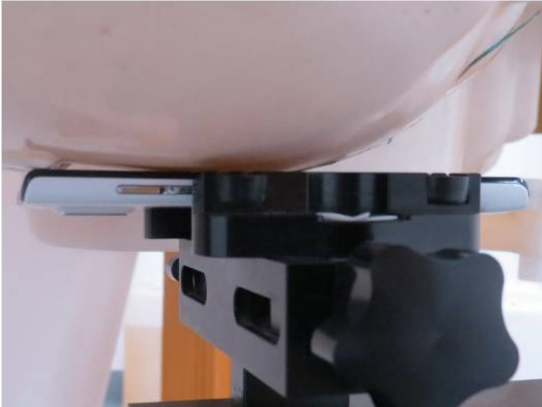
Picture 13: Right Hand Touch Cheek Position
