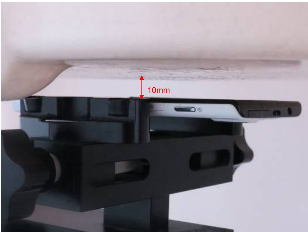
Picture 16: Front Side, the distance from handset to the bottom of the Phantom is 10mm
