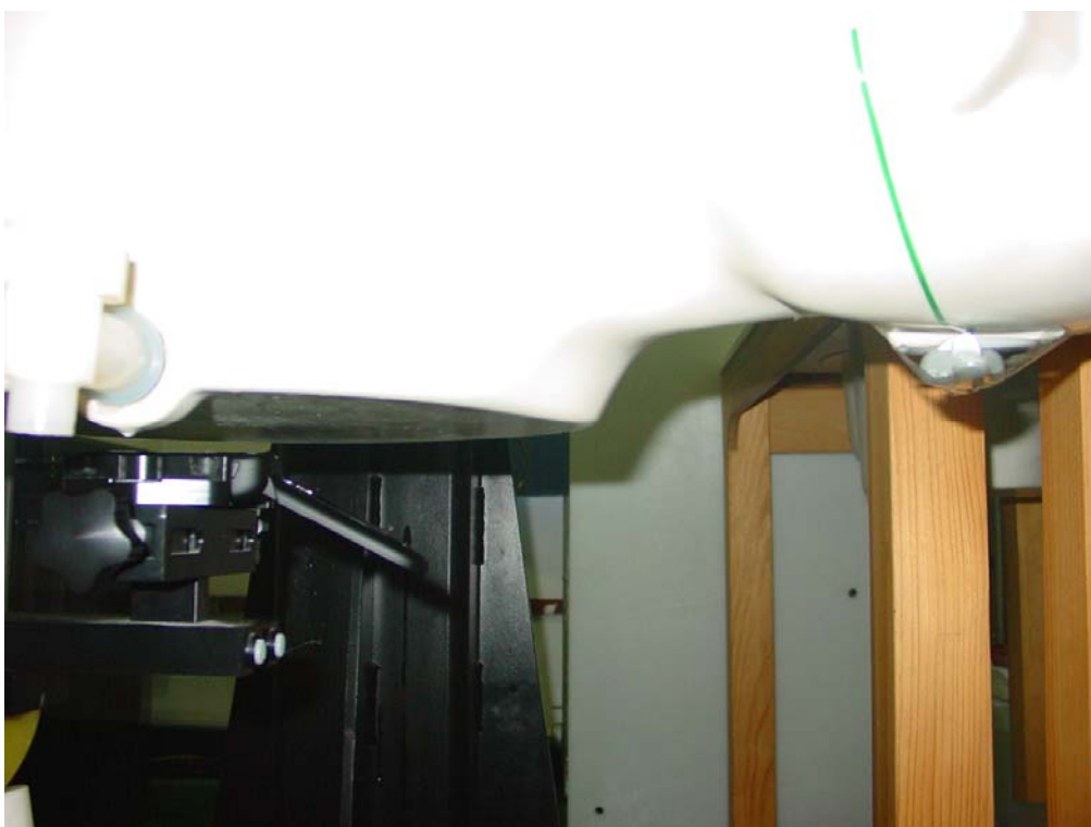
Picture B9: Body-worn Position with Bluetooth (toward ground, the distance from handset to the bottom of the Phantom is 1.5cm)
