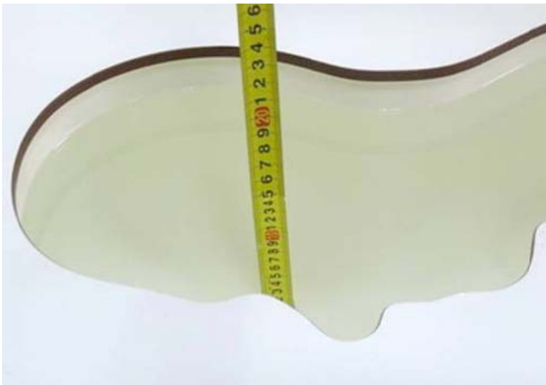
Picture 15: Liquid depth in the head Phantom (5200 MHz, 15.4cm depth)
