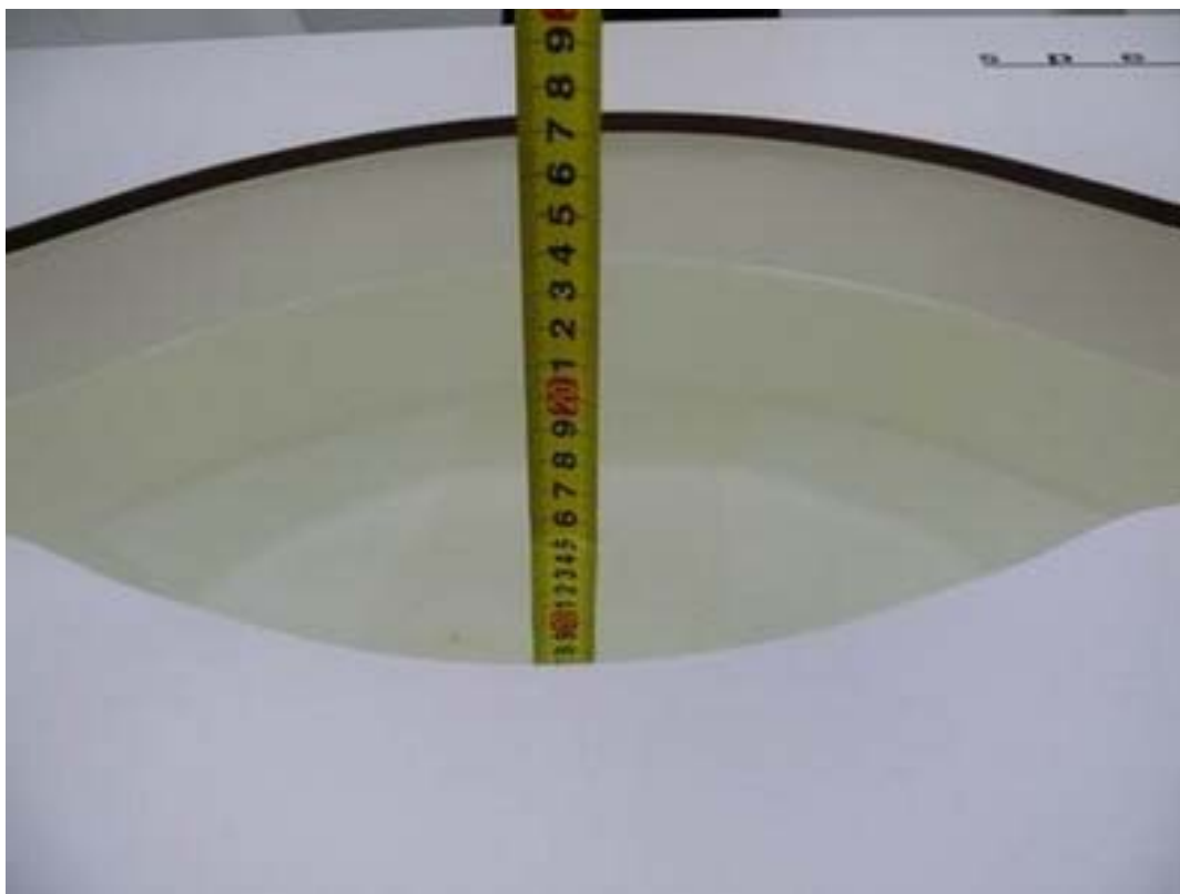
Picture 16: Liquid depth in the flat Phantom (5200 MHz, 15.3cm depth)
