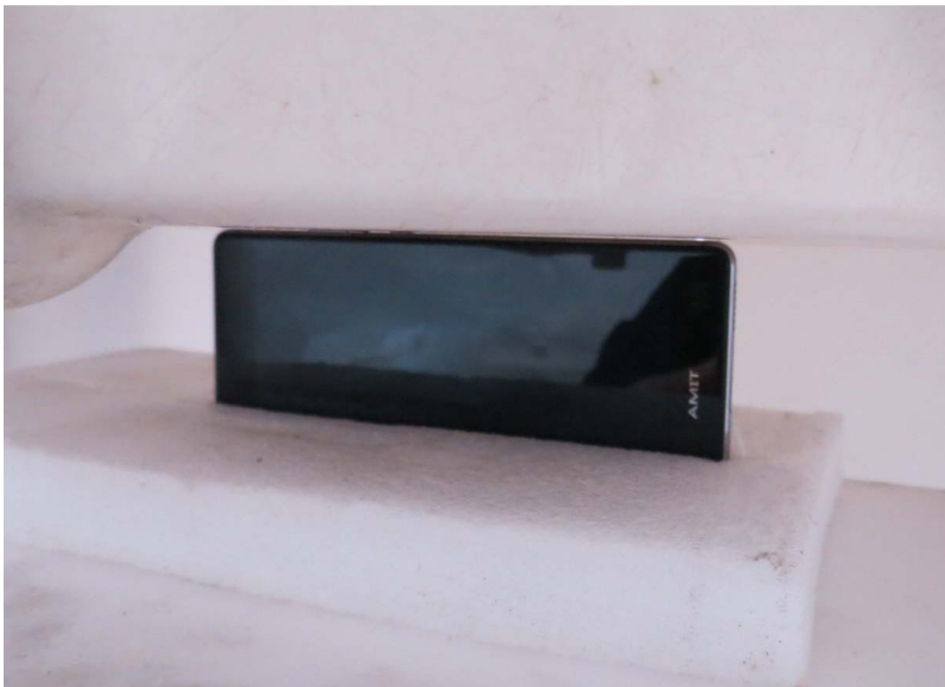
Picture 17: Right Side, the distance from handset to the bottom of the Phantom is 0mm
