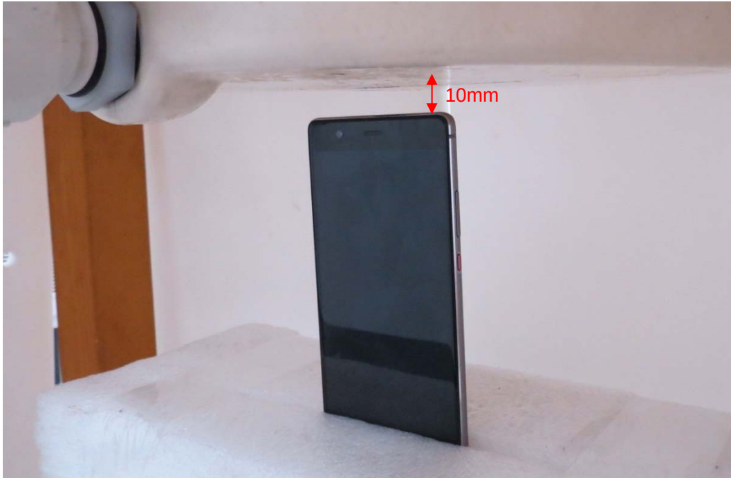
Picture 12: Top Side, the distance from handset to the bottom of the Phantom is 10mm
