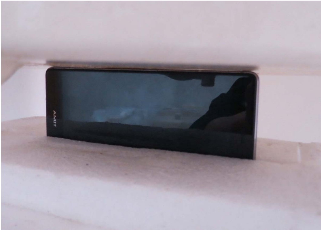
Picture 16: Left Side, the distance from handset to the bottom of the Phantom is 0mm
