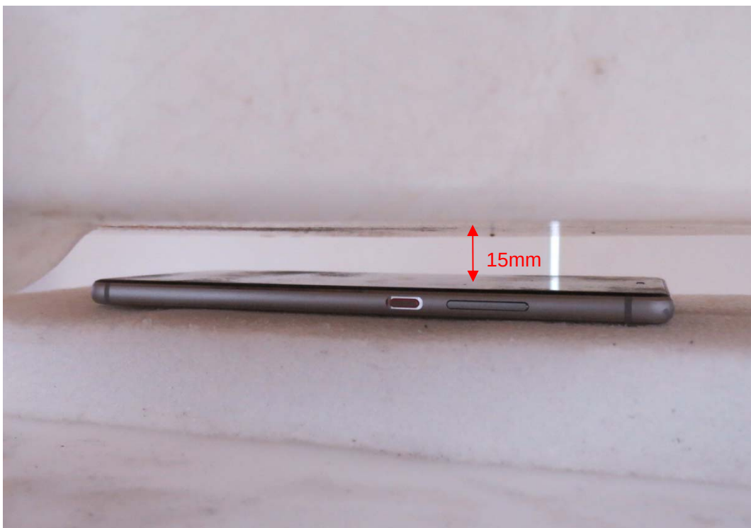
Picture 7: Front Side, the distance from handset to the bottom of the Phantom is 15mm
