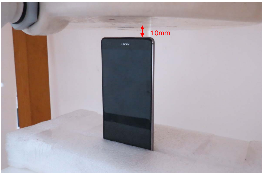
Picture 13: Bottom Side, the distance from handset to the bottom of the Phantom is 10mm
