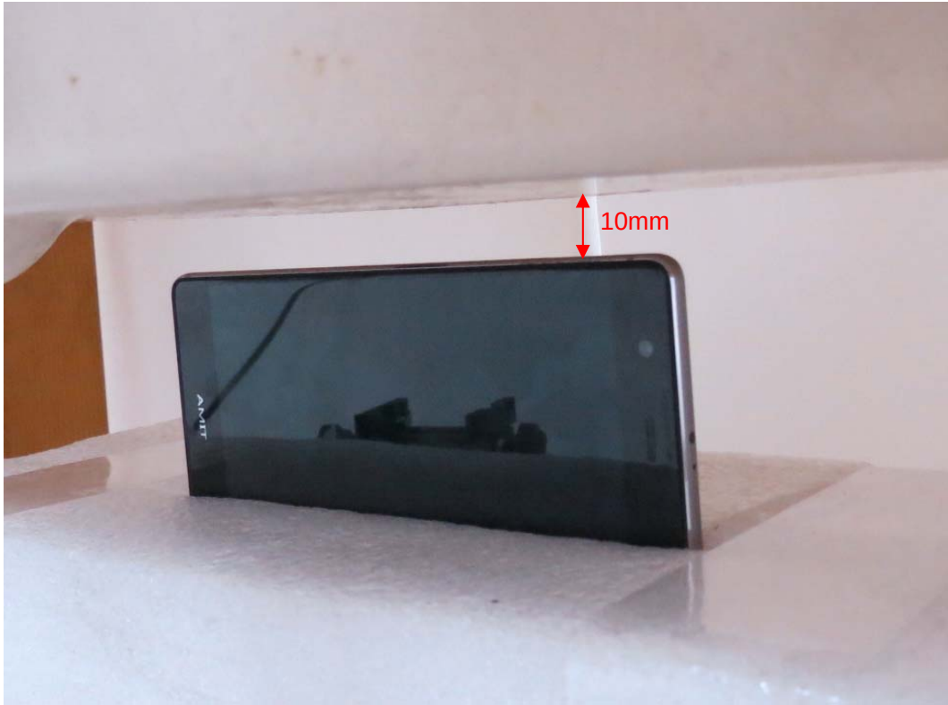
Picture 10: Left Side, the distance from handset to the bottom of the Phantom is 10mm
