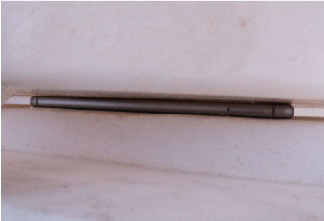
Picture 14: Back Side, the distance from handset to the bottom of the Phantom is 0mm
