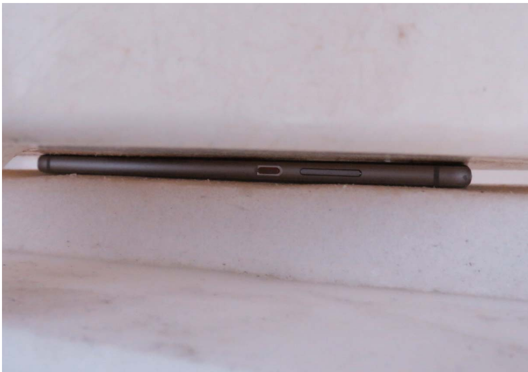
Picture 15: Front Side, the distance from handset to the bottom of the Phantom is 0mm
