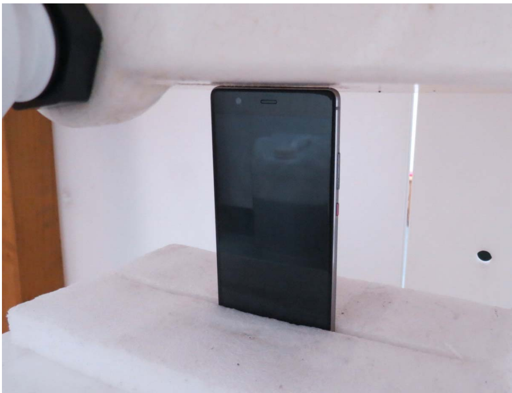
Picture 18: Top Side, the distance from handset to the bottom of the Phantom is 0mm
