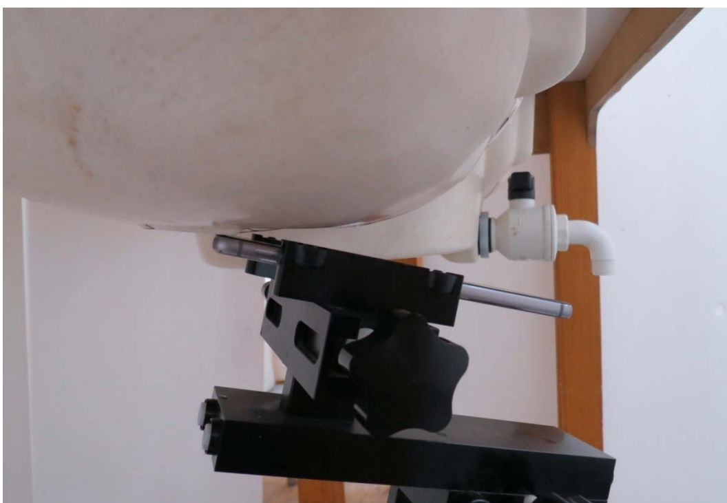
Picture 5: Right Hand Tilt 15 Degree Position
