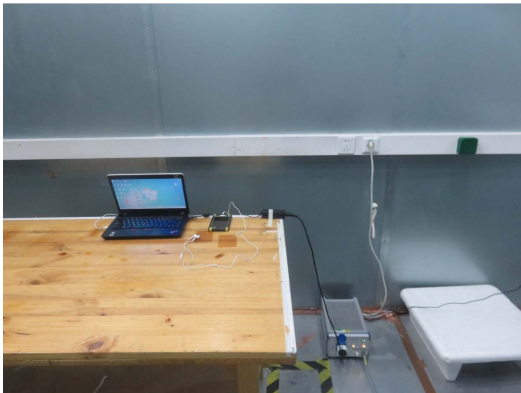
Picture 3 Conducted Emission Test Setup
