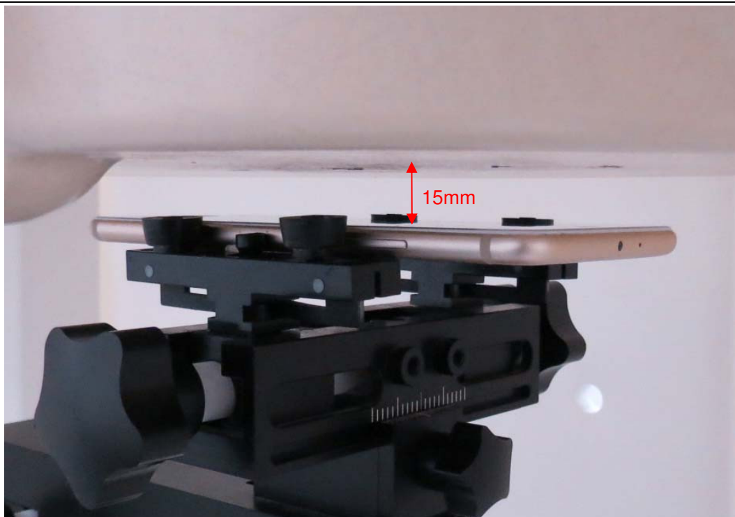
Picture 8: Front Side, the distance from handset to the bottom of the Phantom is 15mm
